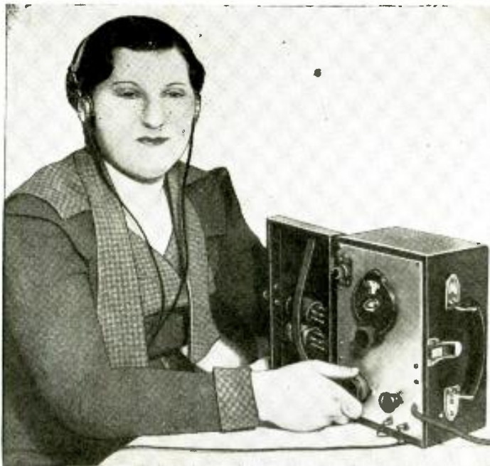
This is one of the most compact and efficient All-Wave portables we have seen—and it works on 110 volts A.C. or D.C.; or with a 6-volt filament battery and two 45-volt "B" batteries.
