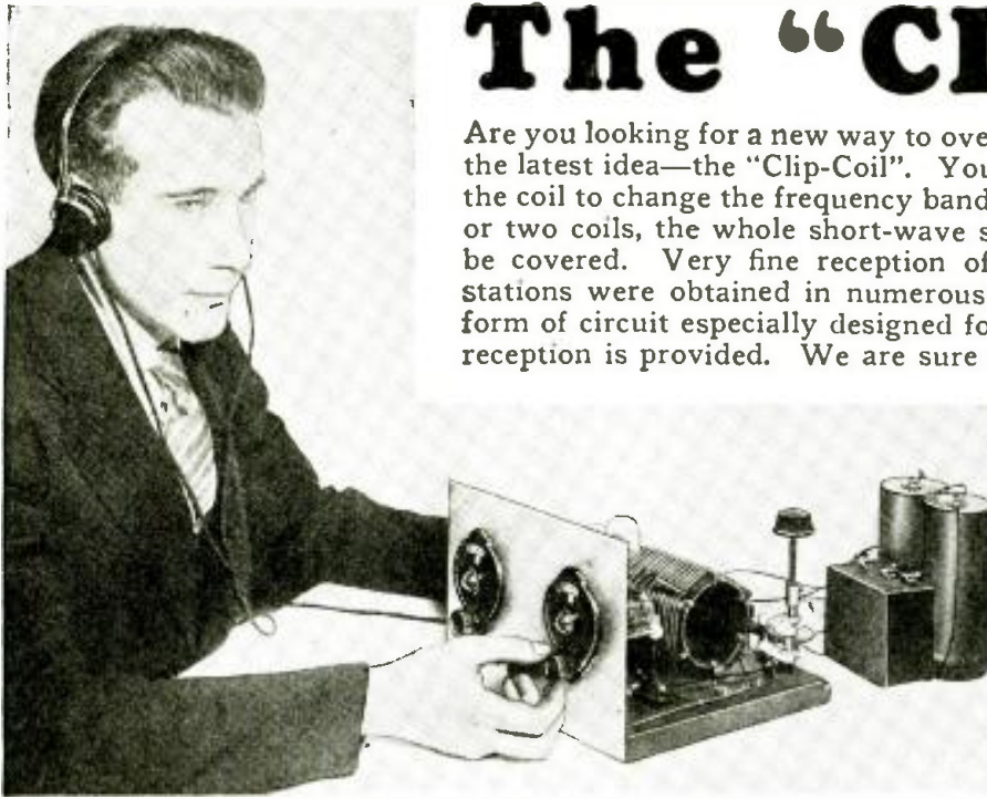
Mr. Stuart takes a whirl at the dials of the "Clip-Coil Two"—a radically different idea in short-wave receivers. The Clip-Coil does away with the need for plug-in coils.
