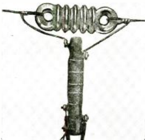
Left—The weather-proofed antenna coupler. Above—Fig. 1, connection of antenna and coupler to feeder line; Fig. 2, details of couplers. Right—The coupler used at the receiving set.
