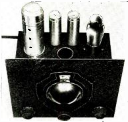
This 2-tube short-wave receiver is really the equivalent of a 3-tube set, a 6F7 "dual-purpose" tube acting as detector and A.F. amplifier. (No. 181.)
