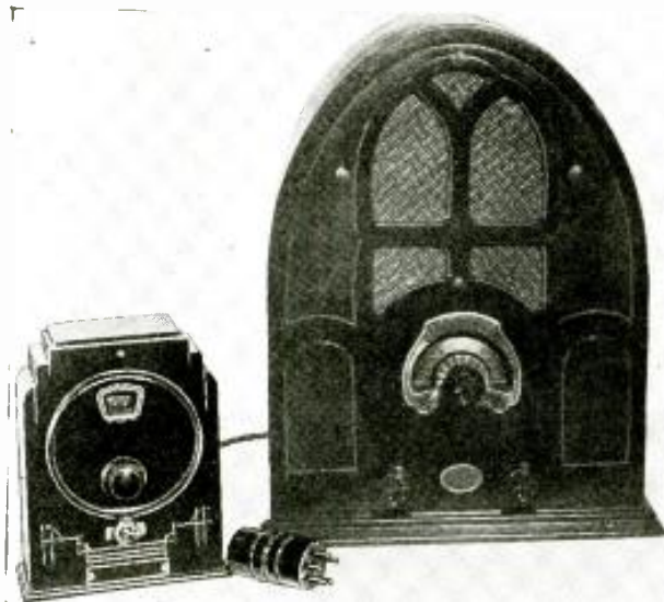
The newest member of the short-wave converter family—the L. C. A. Converter—which enables you to hear "short-wave" stations on your "broadcast" receiver. (176.)
